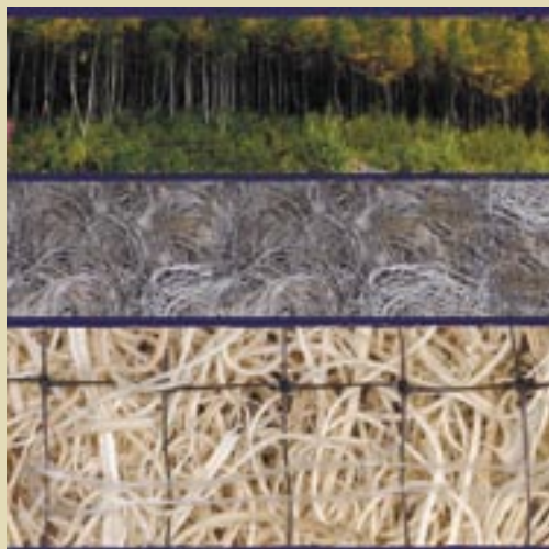
Example of Aspen Trees, Raw Excelsior Fibers and Excelsior ECB
