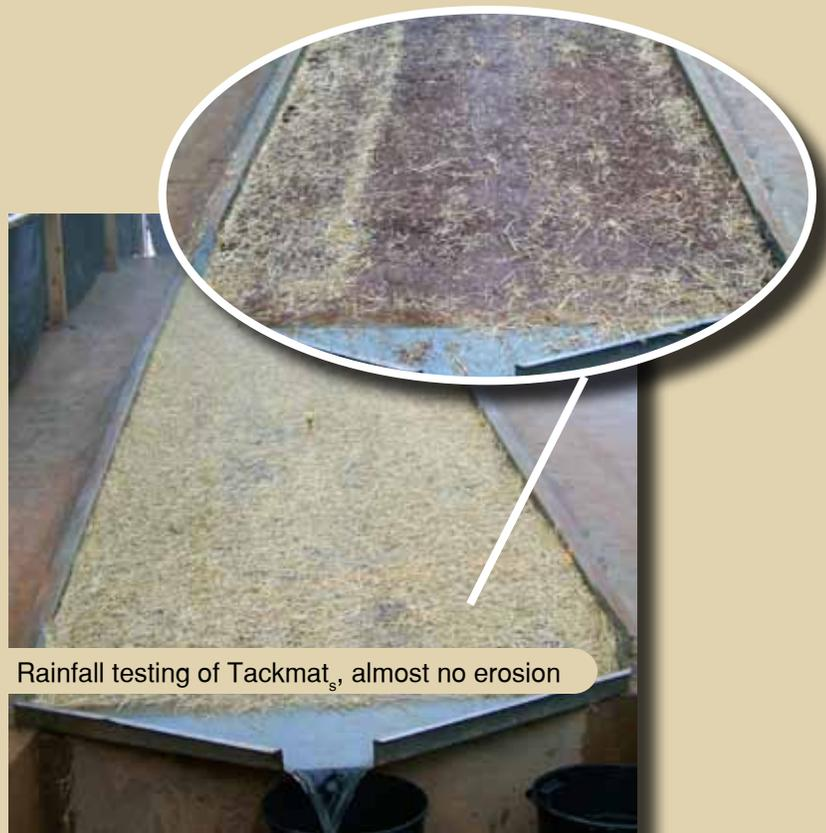
Rainfall testing of Tackmat<sub>s</sub>, almost no erosion
